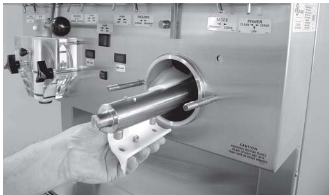
Figure 14. Auger Flight Removal
